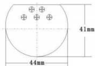
普通型三线制厚度: 18mm Thickness for Normal Type w/ Three Wire: 18mm (含接线端子为22mm) (22mm if including connection End)
