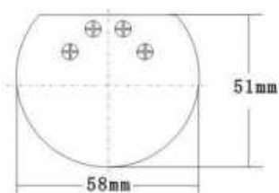
防爆型厚度: 24mm Thickness for Explosion-separation Type: 24mm
